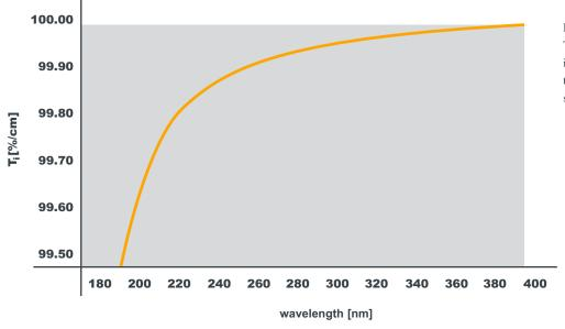
HPFS® ArF Grade is certified to meet  $T_{\rm i} \geq 99.5\%/cm@193nm. \mbox{Higher transmittance}$  is available upon request. A typical internal transmittance curve for HPFS® ArF Grade fused silica is shown here.
